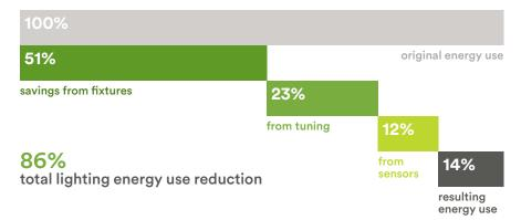
The Neo-Ray fixtures reduced lighting energy use in the *Living Lab* space by 51%. The Encelium controls saved an additional 23% through tuning and 12% through occupancy and daylight sensors. The total reduction in lighting energy use was 86%.
