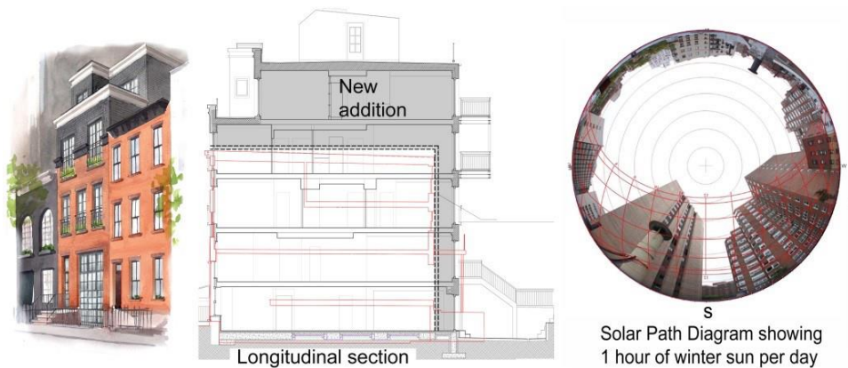
Figure 1: Main constraints: adding 1 ½ stories to a 1910 building and insufficient solar potential
