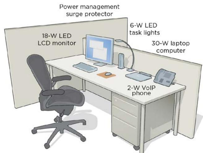
**Figure 5.** Diagram of an example low-energy workstation. Illustration by Matthew Luckwitz, NREL
