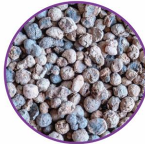
UP TO 50% FLY ASH AGGREGATE IN CAST IN PLACE CONCRETE
