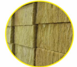
CAVITYROCK INSULATION BY ROCKWOOL R-16 CONTINUOUS AT ABOVE GRADE EXTERIOR WALLS
