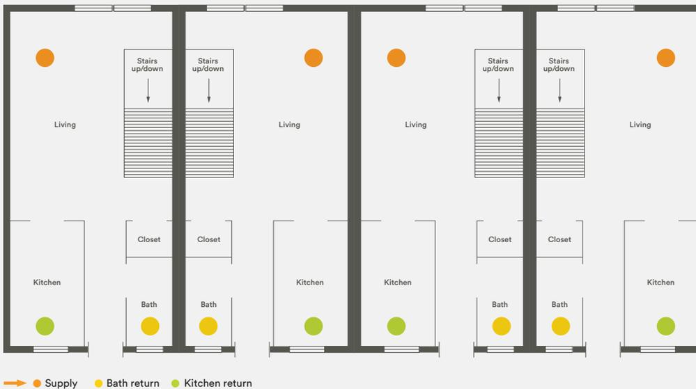
In the proposed scenario Individual ERVs are provided for each apartment, usually requiring two penetrations through the exterior wall per apartment. Exterior ERV units may be hung near the ceiling or exterior wall, or potentially on balconies if available.
