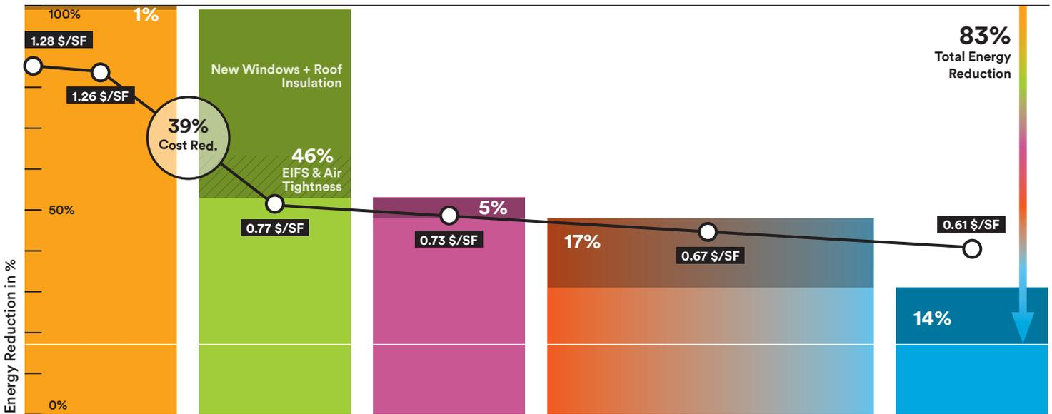
Because the building envelope plays such a critical role in heating demand and overall comfort, additional wall and roof insulation, improvements to airtightness, and the introduction of high performance windows have the greatest impact on energy use, utility cost, and carbon emission reductions.
