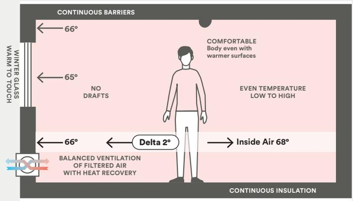
Insulating the exterior walls and installing high-performance windows ensures that the inside surface temperature of the exterior walls remains warmer throughout winter and, most importantly, closer to the interior air temperature. Research indicates that comfort is significantly compromised when this difference is greater than 7 degrees F. We estimate the existing building suffers from a difference nearly 3x this figure.
