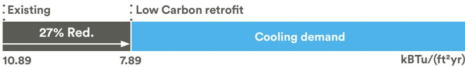
Although a high performance envelope does not reduce the cooling demand nearly as much as the dramatic reductions in heating demand, reduction in cooling demand by 20-30% remains extremely important as that reduction will occur during periods of peak demand for electricity—periods when utility costs and carbon penalties are likely to be highest in the future.
