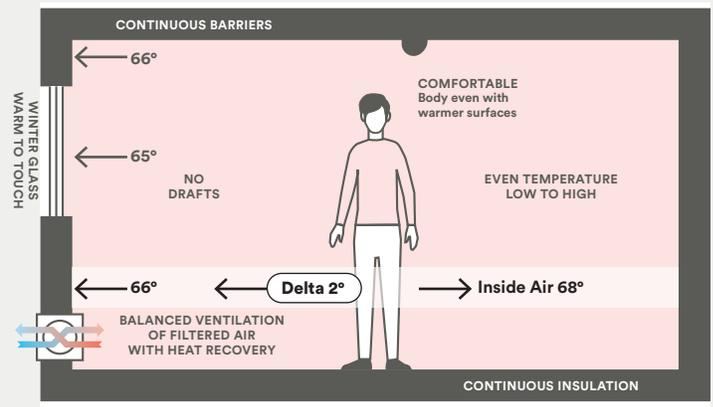
Insulating the exterior and installing high-performance windows ensures that the inside surface temperature of the exterior walls remains warmer throughout winter and, most importantly, closer to the interior air temperature. Research indicates that comfort is significantly compromised when this difference is greater than 7 degrees F. We estimate the existing building suffers from a difference nearly 3x this figure. Graphic credit: Building Energy Exchange
