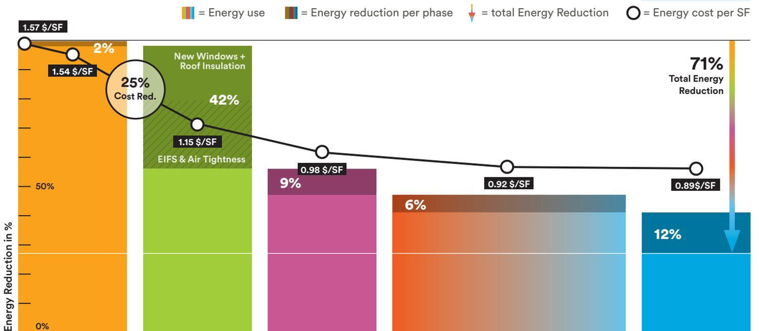
Because the building envelope plays such a critical role in heating demand and overall comfort, additional wall and roof insulation, improvements to airtightness, and the introduction of high performance windows have the greatest impact on energy use, utility cost, and carbon emission reductions.
