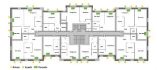
The preferred VRF option limits interior construction by placing the new refrigerant lines on the outside of the existing masonry walls and directly accessing the new cassettes over each window
