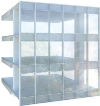
6: After Complete Removal of Old Facade
