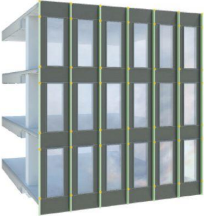
2: Install Clips to Attach New Facade
